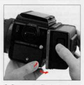
C. Depress the film back release button and the lower end of the film back can be removed, as illustrated. Simply shift the film back up slightly and pull it away.
