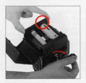
E. The starting point, or arrow mark of the unexposed film, can also be aligned with the start-mark, with the film insert loaded in the film back. Simply rotate the film winding crank on the main camera body. This method is preferred since there will be coupling with the main camera body mechanism, from the beginning.
