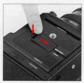
A. Depress the battery chamber button and, at the same time, move the battery chamber cover in the arrow-indicated direction. The cover will come off easily.
