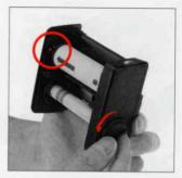
D. Rotate the film back winding crank on the right side of the film insert in the direction indicated by the arrow, while checking the advancing film.
