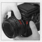
B. To detach the lens, the film winding crank must also be rotated to cock the lens shutter first. Then, press the lens release button down and, at the same time, rotate the lens in the clockwise direction until it makes a full stop, at which point it will be possible to detach the lens.
