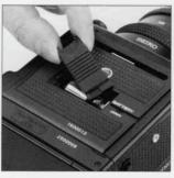
B. Coincide the plus (+) and minus (-) marks on the battery with similar polarity indications in the battery chamber. Then, push in the battery. Insert the battery chamber cover into the "BATTERY" end first and then move the cover in the other direction (opposite to the arrow indication) until it locks.
