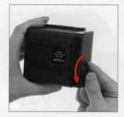
H. The manual film winder is used for advancing the film, when the film back is detached from the main body for film loading. The manual film winder can continue to rotate, even when the film is set for the first exposure. It should be rotated 2 or 3 times more, in order to take up any slack in the loaded film.
