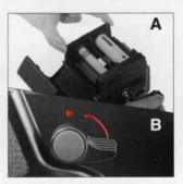
\* If the film is not advanced when the film winding crank is rotated, the film holder is not inserted properly (A) and/or the main camera body may be set for multiple exposures (B). In the latter case, return the multiple exposure lever to an upright or vertical position. (See "22. Multiple Exposures" on
