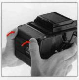
F. Close the back cover, by pressing it firmly against the base of the film back, as illustrated. The back cover will automatically close and lock.
