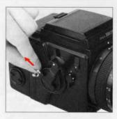
The film winding crank can be detached by pulling out the crank shaft as illustrated and the Speed Grip S may be attached in its place. For use, see instructions supplied with the Speed Grip S.
