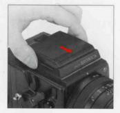
A. The waist-level finder can be interchanged, with other optional finders, to match shooting conditions with photographic conditions. To attach the finder, align the front end of the finder frame on top of the camera main body, as shown. Then gently lower the finder and, when well-seated, slide forward until it locks.
