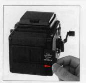
Upon loading the film tear off the end flap from the empty film package and insert it in the film type indicator frame. This will help you keep track of the film loaded in the film back, even when two or more film backs are used with different films.
