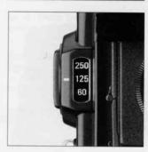
The number on the shutter speed scale indicates the set shutter speed. For example "8S" is 8 sec., "2S" is 2 sec., "2" is 1/2 sec. and "500" is 1/500 sec. Intermediate speed settings are not available.
