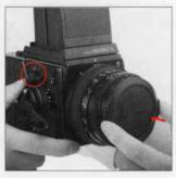
a. Cover the lens and take one blank exposure, as follows: First, return the mirror lock-up switch lever to N setting. Then, use the multiple exposure lever and expose the frame. Finally, after exposing the frame, reverse the multiple exposure lever.
