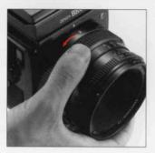
A. To attach the lens to the main body, align the orange dot on the main camera body and the red dot on the lens, and then insert the lens fully into its mount. Rotate in the counterclockwise direction until it stops, with an audible click, which will indicate that it is securely locked
