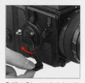
E. When C is set to the index, with the mirror lock-up switch lever, the lever will not return to N, with the next film advance and shutter cocking action. Therefore, shooting with the mirror locked up will be possible any number of times.
