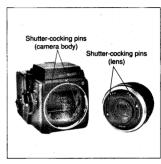
• Both main camera body and lens must be in the "cocked" condition to attach or remove the lens. In other words, when "cocked" the cocking pin of the lens will be set between the red band and green dot, while the cocking pin of the main body mount will be set to the green colored dot
