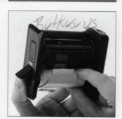
After completing exposing one roll of film (12 exposures), continue winding until the leader paper is completely wound up, or approximately 8 full turns of the advance crank. Then, open the back cover and take out the film holder.
