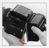
A. To attach the film back to the main camera body, simply insert the latches at the upper end of the film back into the attachment openings at the upper end of the main camera body. Then, press the lower end of the film back against the main body until it locks securely.
