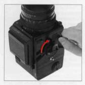
G. Upon loading the film, rotate the film winding crank until it stops to place the first frame into place for taking the picture. The exposure counter will also change from "S" to "1", while the shutter will also be cocked.
