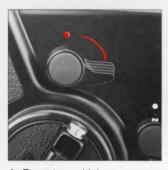
A. To make multiple exposures, rotate the film winding crank (to advance the film and cock the shutter). Turn the multiple exposure lever in the clockwise or arrow-indicated direction, which will expose a red mark. When set in this manner, the shutter can be released and cocked any number of times, without advancing the film.
