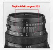
depth-of-field scale is next to the distance scales and is made up of identical pairs of apertures on both sides of the orange-colored distance index. These identical pairs of apertures indicate the distance zone in focus at these lens openings. For example, if the 80 mm lens, stopped down to f/22, is focused at a distance of 3 m (10 ft), the depth-of-field scale shows that the zone will extend from 2 to 7 m (7 ft. to 23 ft.) at f/22.
