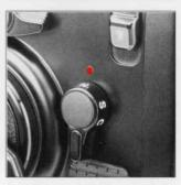
A. The mirror lock-up switch lever has three settings, or N, S and C, with the lever rotated to set N (normal) to the index for shooting without locking up the mirror and to S (single frame) or C (continuous) for shooting with the mirror locked up.
