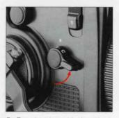
B. For shooting with the mirror locked up, first, cock the shutter. Then, rotate the mirror lock-up lever in the arrow-indicated direction and coincide S or C to the index. The lens shutter will close completely and the reflex mirror and film safety plate will swing up.
