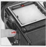
If a red-colored battery check LED lights up outside the focusing screen area (central front of finder), when the battery check button is pressed, the battery is loaded properly and there is sufficient power for operations.
