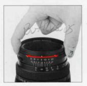
A. The aperture ring is rotated, in either direction, to set the required f-number opposite the white index dot. The aperture ring click-stops at Intermediate settings are also possible.
